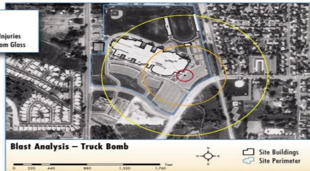
Figure 4-7 Blast analysis of a building for a typical large truck bomb detonated in the building's parking lot
