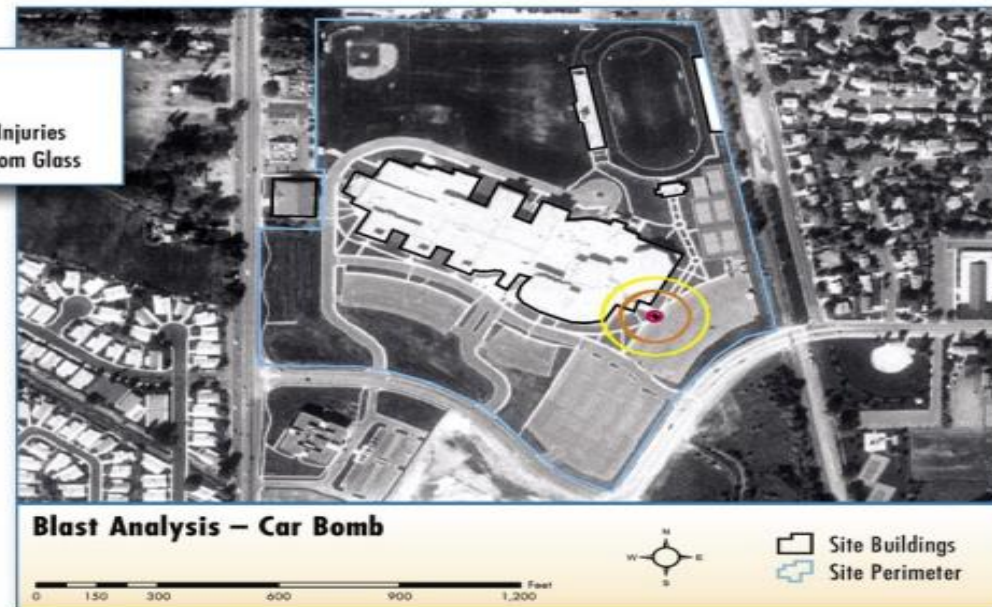
Figure 4-6 Blast analysis of a building for a typical car bomb detonated in the building's parking lot
